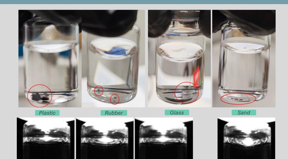
The dataset was acquired internally by *Performing Beyond Limits (PBL)* and consists of 2,426 vial sequences filled with water, with 19 frames each. It includes **five different classes**: one represents the absence of impurities, while the others correspond to four foreign particles: burnt plastic, rubber particulates, glass fragments, and sand debris.
